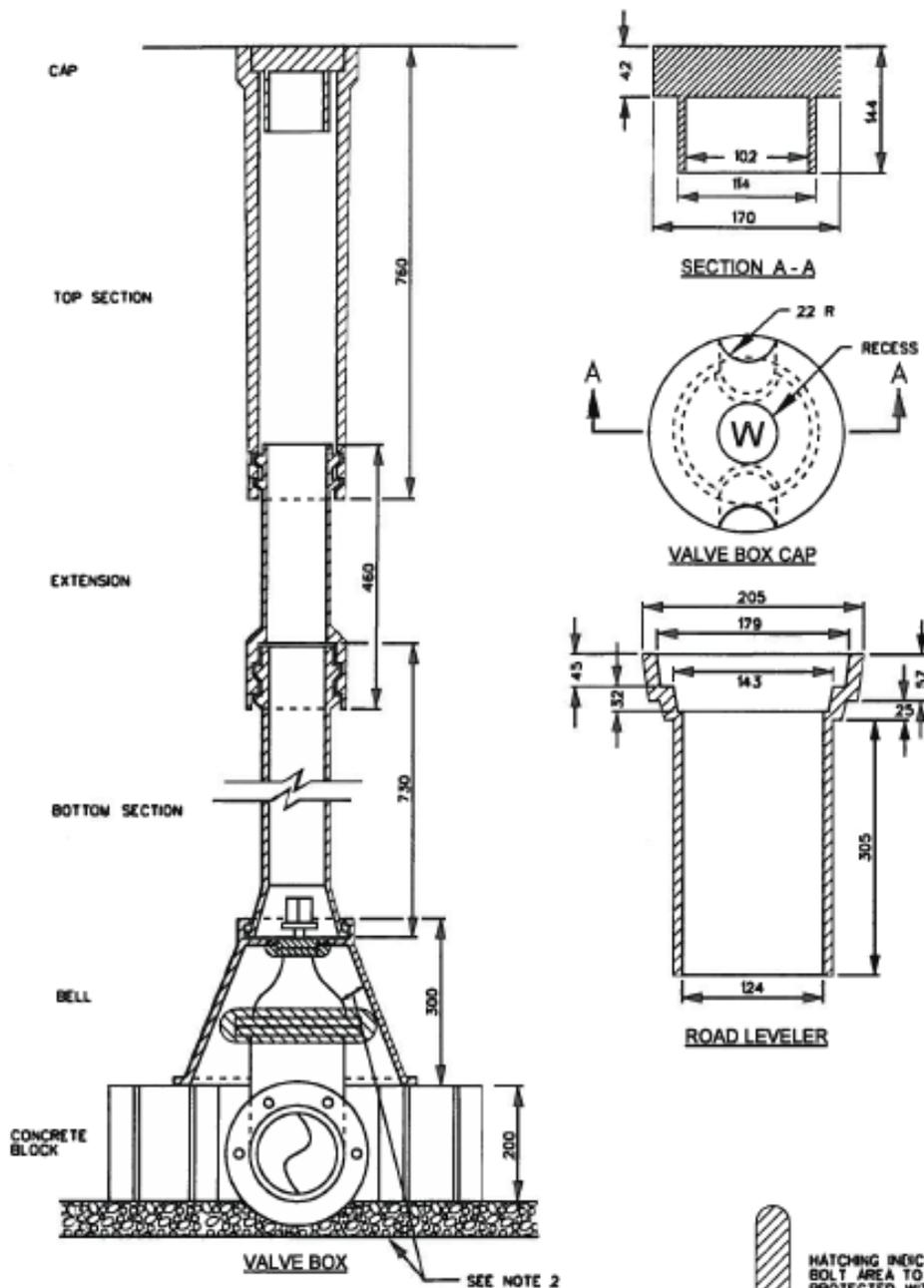
HATCHING INDICATES BOLT AREA TO BE PROTECTED WITH AN APPROVED PETROLATUM TAPE SYSTEM
